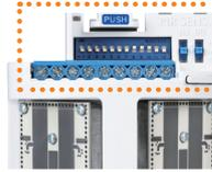
All the components needed for the sensor's adjustment and settings are in blue.
